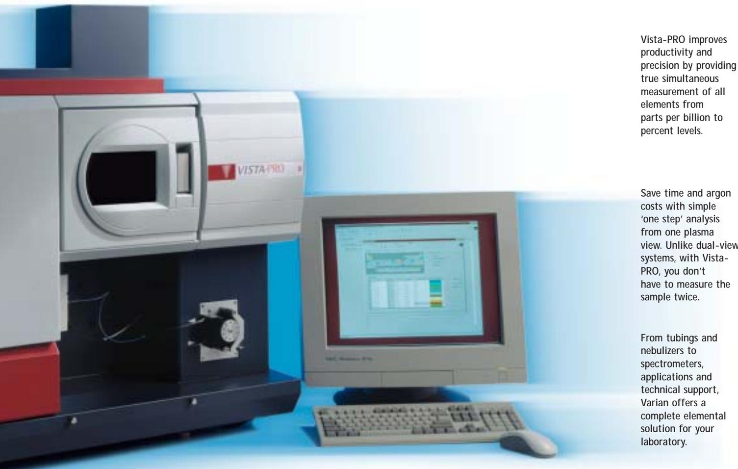
Vista-PRO improves productivity and precision by providing true simultaneous measurement of all elements from parts per billion to percent levels.
