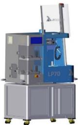
The LP70 is a multi-station precision lapping and polishing machine, which runs concurrent automated processes, achieving repeatable results to stringent sample specifications. In order to keep this machine in optimum condition, please read the following operation and maintenance information, and have the manual available to all operators of the machinery. Regular cleaning and basic maintenance of the machine will extend its life.
