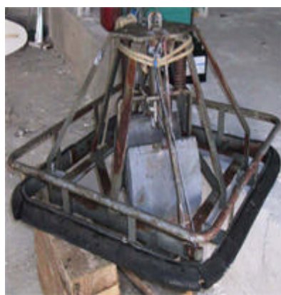
11. Benne Smith & Mc Intyre (100 kg)
